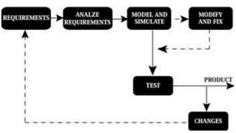
Figure 2–1: Modeling and simulation process
